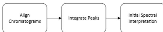
Figure 1: Framework of a typical E&L data processing workflow
