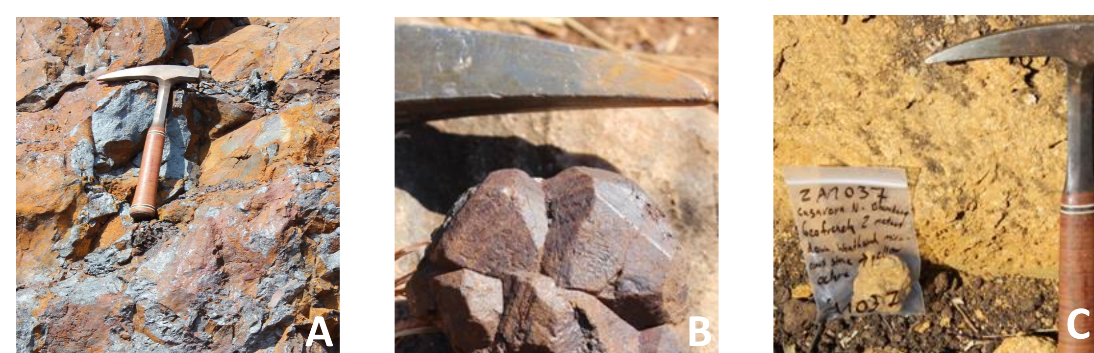
Figure 1. A: Massive specular hematite B: Martite habit of hematite C: Ochreous yellow clay weathered from mica D: Red and yellow ochreous shale E: Ochreous red clay from igneous rock hydrothermally weathered
